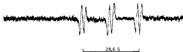
Figure 1. The first derivative of the epr spectrum obtained by heating \alpha,\alpha -diphenyl- N -benzhydrylnitron above 100^\circ in diethyl Carbitol.
